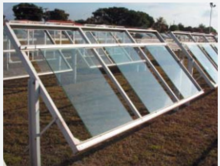
Fig 4: Samples of laminated glass at the DuPont weathering Site, Hialeah Florida.
