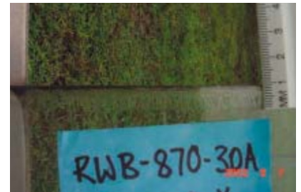
Fig 6: Open edge of a Type X laminate after 54 months of Florida exposure
